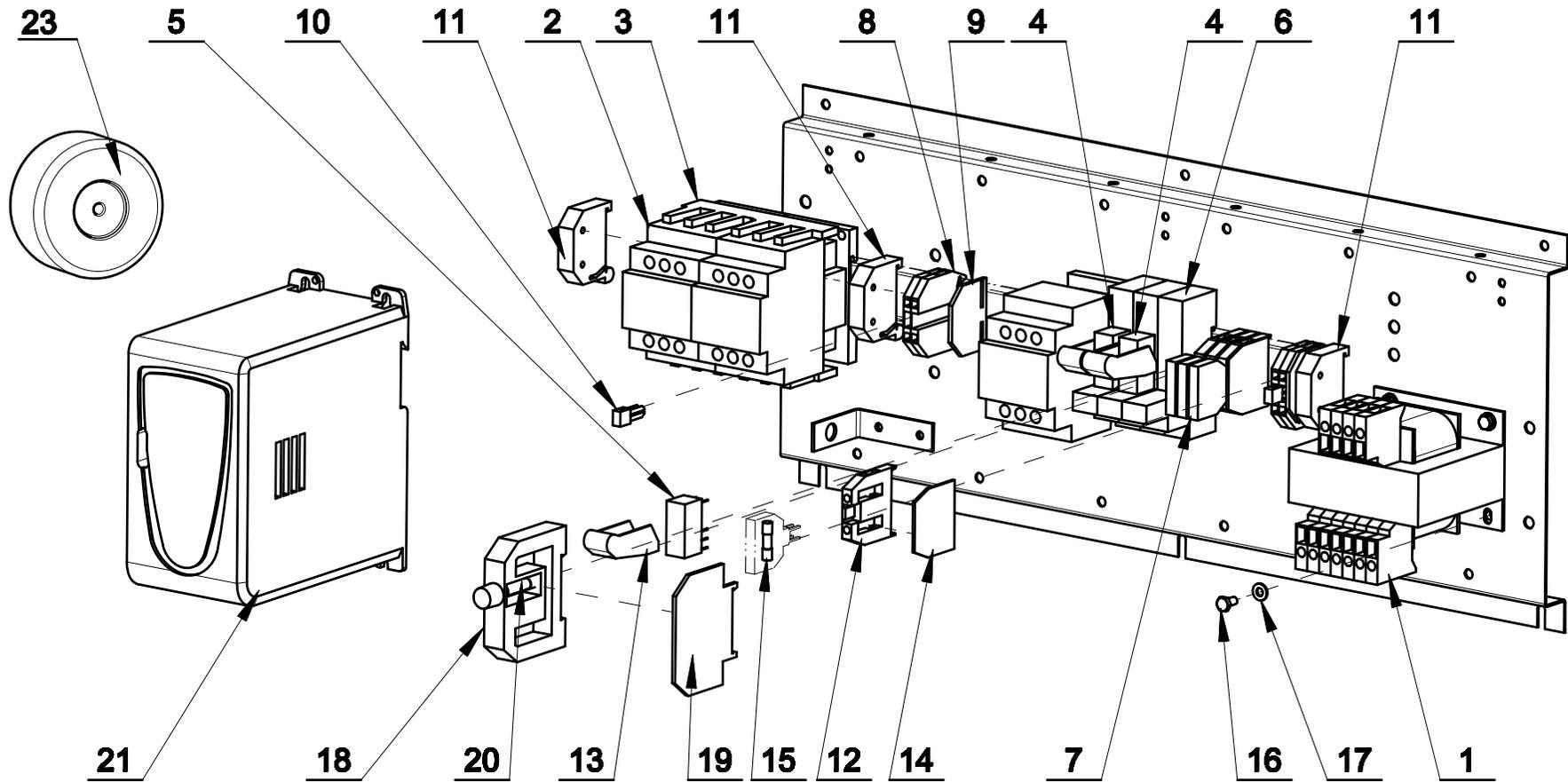
**Box of electrical components for gas and steam heating: drawing nr. 520512 B**
